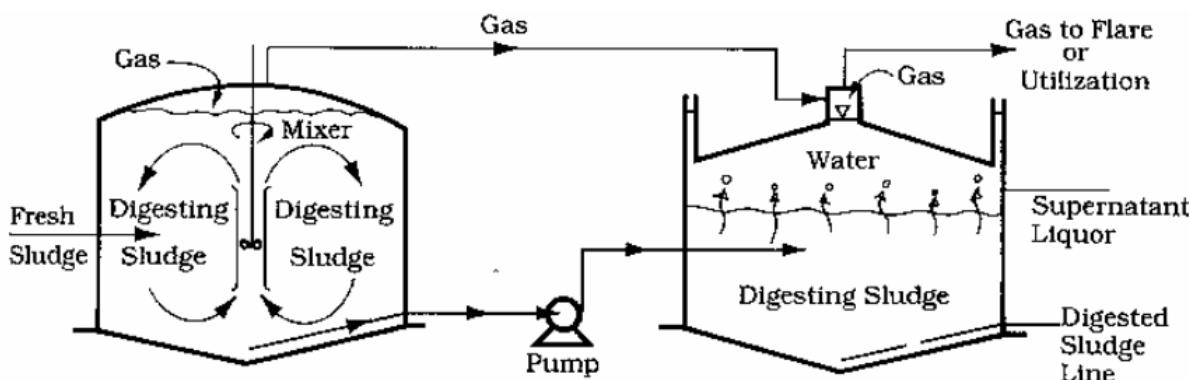
Figure 1 - Two-Stage Mesophilic Anaerobic Digester Process Flow Diagram
