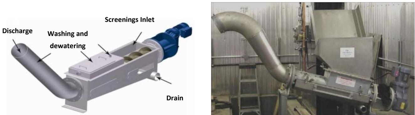
Figure 6      ROTOPAC RPW pretreatment (dewatering, washing and compacting)
