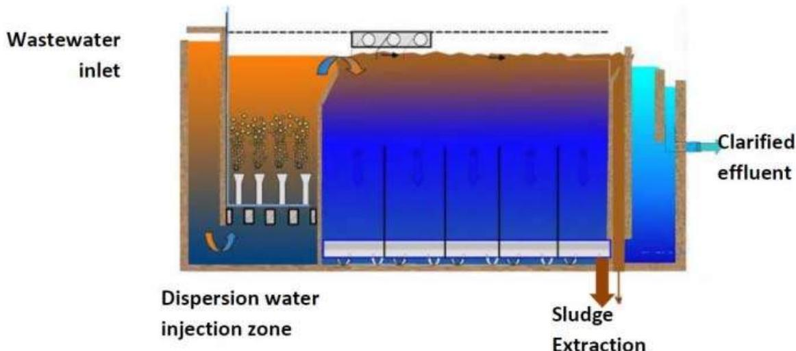
Figure 4 - Spidflo® Process Diagram from Veolia
