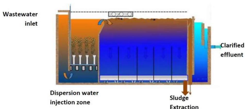
Figure 5 Spidflow Secondary clarifier
