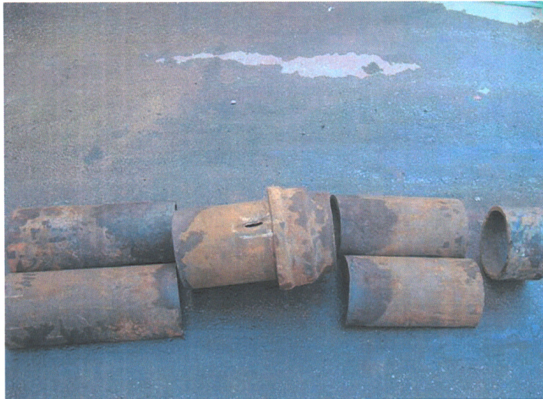
Image 23 – Pipe Sample after Sectioning
