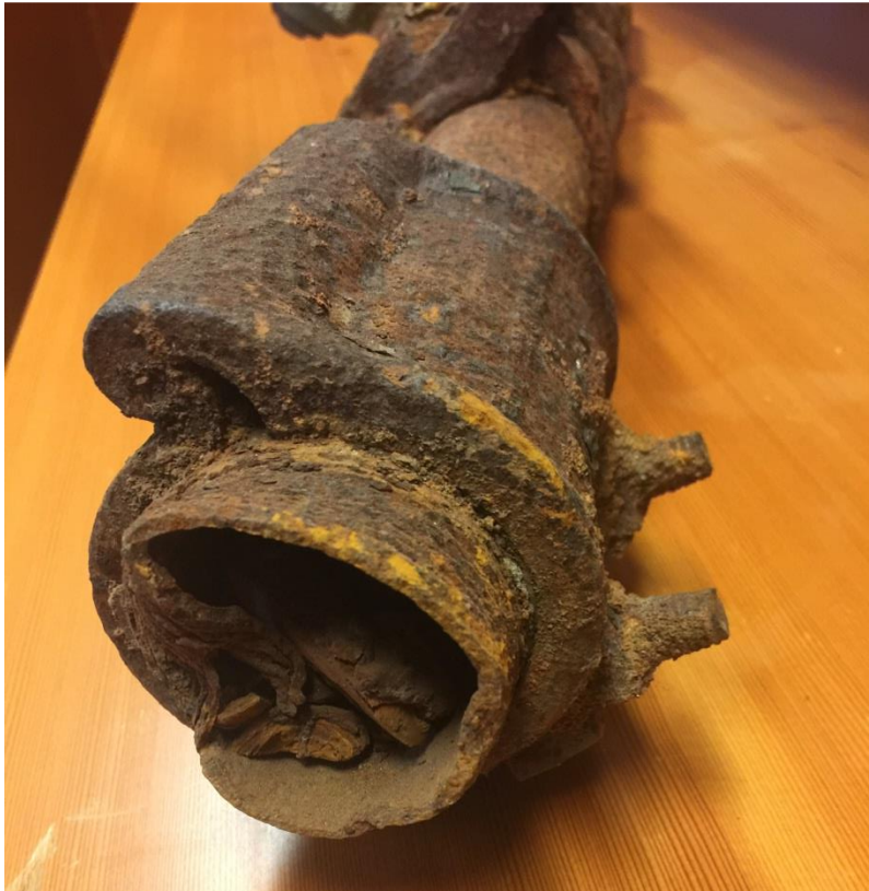
Sample of corroded galvanized pipe replaced throughout Nelson.
